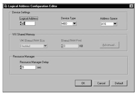
Figure 6-3. PCI-MXI-2 or PXI-MXI-2B Logical Address Configuration Editor
